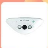
MVT-D30 6mm lens, 24pcs×Ø5 IR leds
