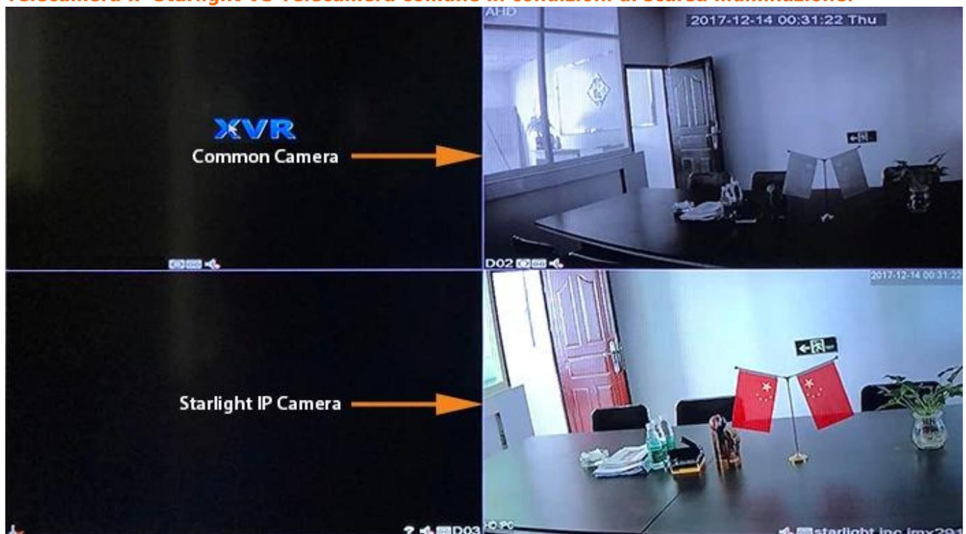
The image shows a side-by-side comparison of two camera feeds in a dimly lit room. The top feed, labeled 'XVR Common Camera', shows a very dark and grainy image where details are lost. The bottom feed, labeled 'Starlight IP Camera', shows a clear, bright image of the same room, demonstrating superior low-light performance. Both feeds include a timestamp '2017-12-14 00:31:22 Thu' and a camera ID 'D02'.
